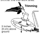
SCALPING - The scalping technique removes unwanted vegetation down to the ground. Hold the bottom of the trimmer head about 3 inches (8 cm) above the ground and at an angle. Allow the tip of the line to strike the ground around trees, posts, monuments, etc. This technique increases line wear.
